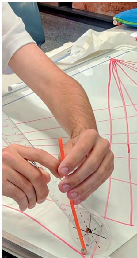
▲ A student calculating the probability amplitude of photons coming from two slits at different points. Using small phasor wheels on white boards, students can find the resultants at different points and calculate the probability amplitude. The square of the probability amplitude is proportional to the number of photons coming at a point per unit time.
