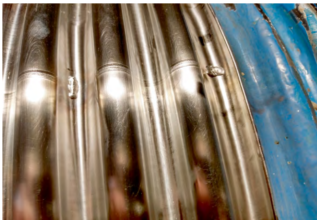
The welding seam to seal the leak.
