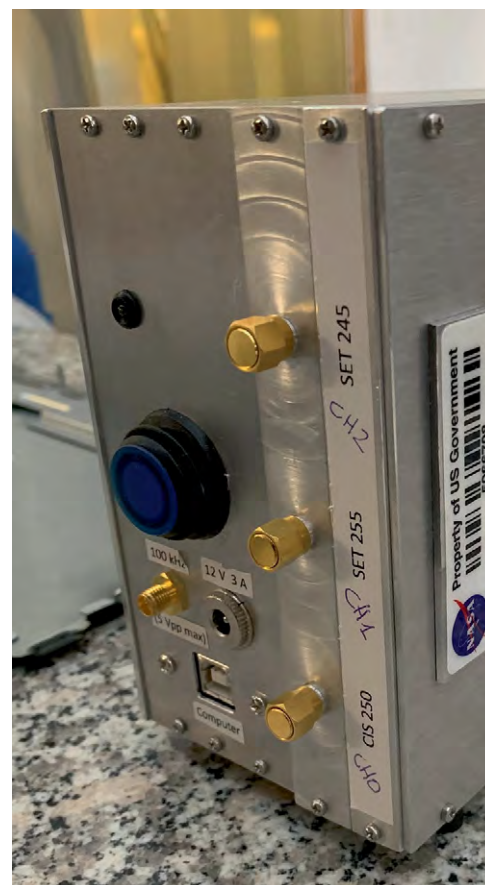
TRL4 prototype CMD, developed by the Precision Space Systems Lab at the University of Florida, delivered to the University of Trento for GRS subsystem-level testing.
